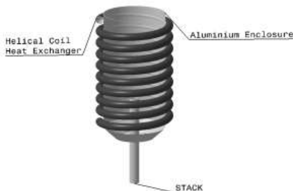
Fig 8 Schematic of a device to extract energy from gas flares.
